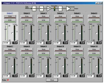
Figure 3.41. Outputs 1-12 configuration window
